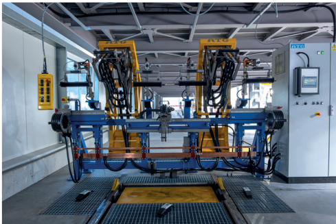
UNIMAG WST – wheel set MPI testing
