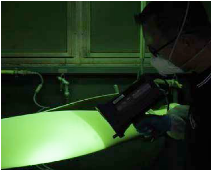
Inspection of propellers by FPI
